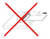
2) Do not add the load mating FPC/FFC with connector housing.
